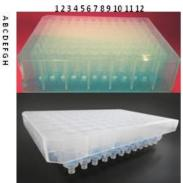
Each well contains a silica-based membrane (Secured by a Red O-ring) (Secured by a Blue O-ring)
