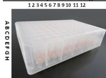
Each well contains a silica-based membrane (Secured by a Red O-ring)
