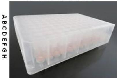
Each well contains a silica-based membrane (Secured by a Red O-ring)
